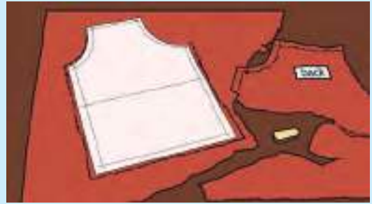
Figure 7.10: Uneven marking and cutting of fabric
