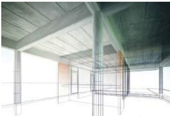
Figure 2.2: Beams support the roof; more weight can be placed over beams compared to the rest of the roof.
