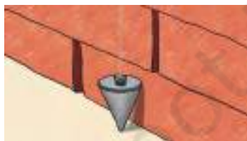
Figure 6.17: (a) Plumb bob must hang parallel to the ground; (b) bubble in spirit level tube must be at the centre; and (c) level in water level tube must be the same at all points of the structure
