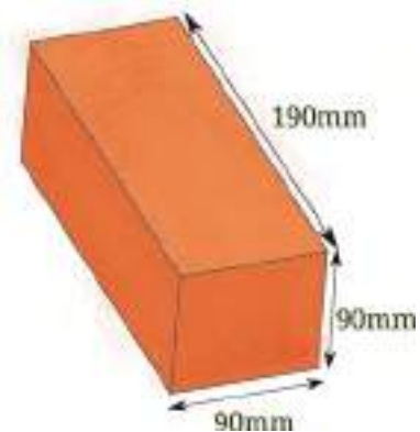
Figure 6.9: Dimensions of a typical brick in India are 190 \times 90 \times 90 mm
